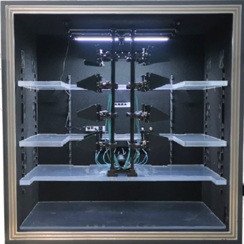
Custom 110cm tall chamber with special antenna mount and shelves
